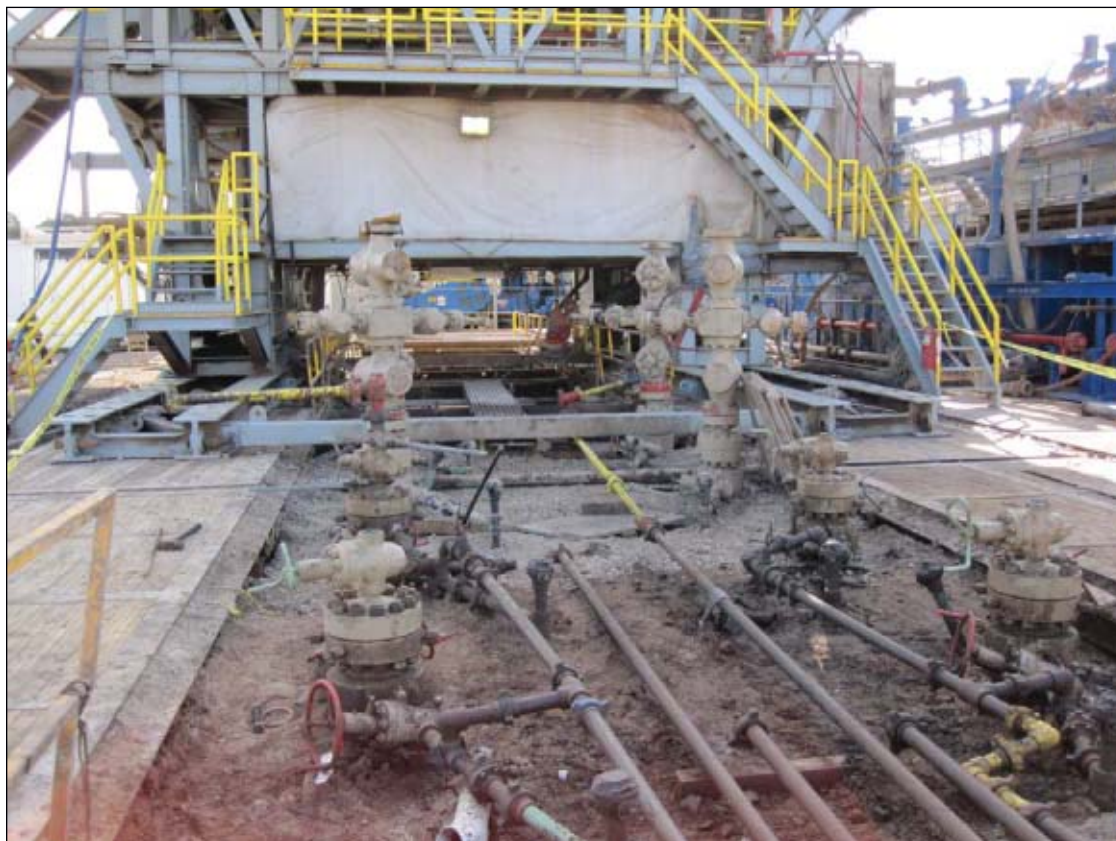
Wells on this pad have a spacing of 7½ ft between wells and 10 ft between rows (Fig. 2). Photo by Guntis Moritis.
