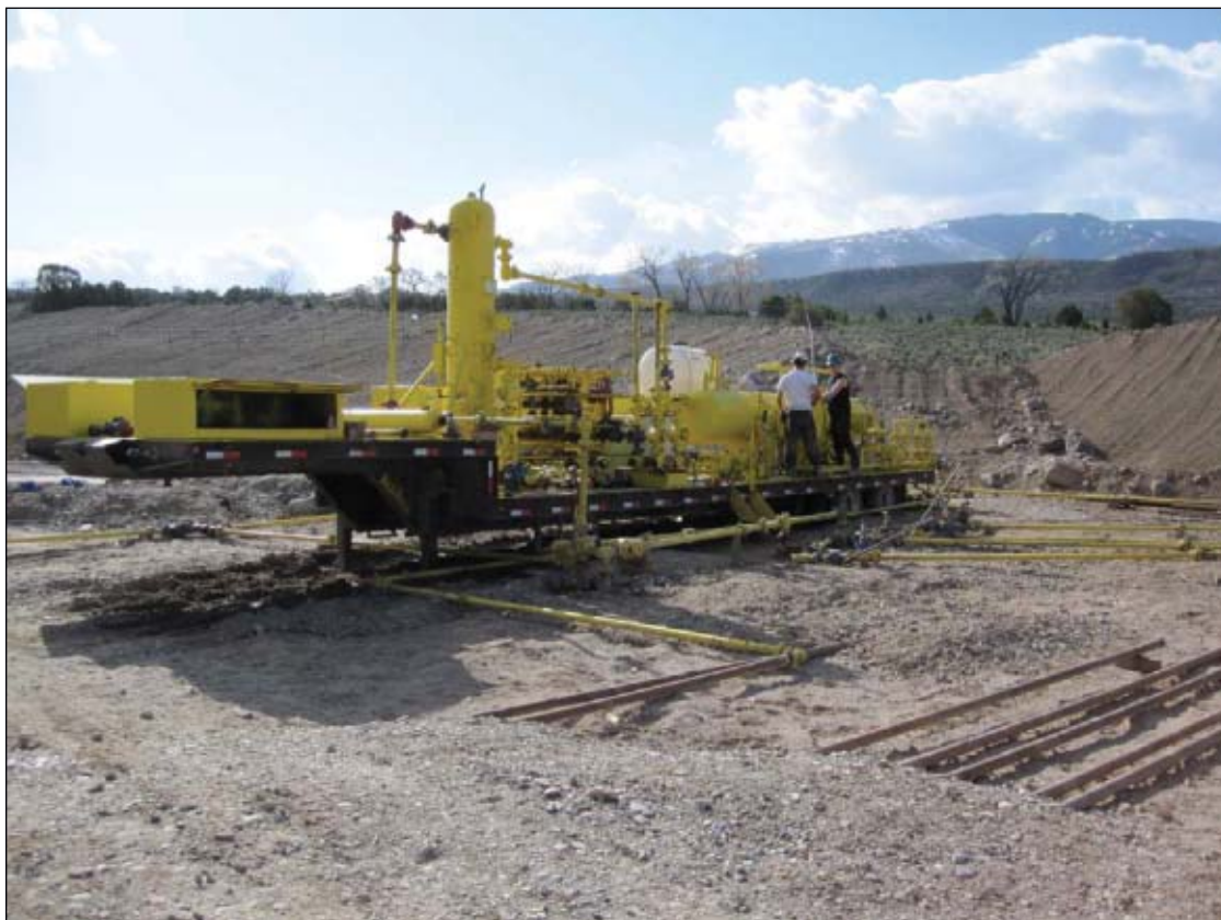
For handling the fluids and sand flowing back after a frac job, Williams uses a skid-mounted separator (Fig. 4). Photo by Guntis Moritis.
