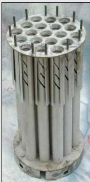
Shown (left) is the ProSep axial flow cyclone bundle and (right) the fully assembled demister (Fig. 1).
