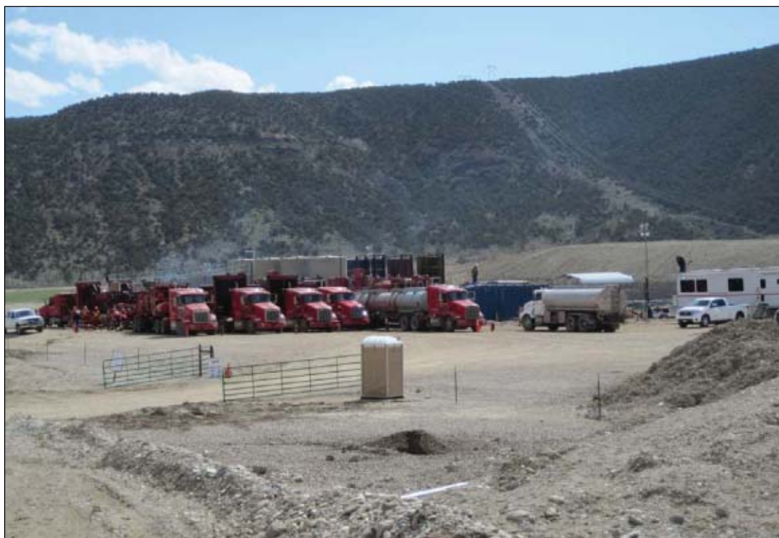
This centralized frac site in South Rulison field has six 2,000-hp frac trucks for a total of 12,000 hp, and a 77,000 bbl water pit in back of the site (Fig. 3). Photo by Guntis Moritis.
